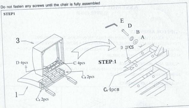
Attach the Seat Frame (3) to the Back Frame (1) using four Flat washer (A), Four Spring Washer (B), and four Bolts (C), with the procided Allen Wrench(D).
